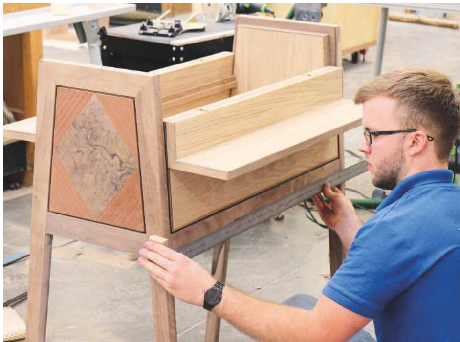
Final checking of overall measurements; note the block stop
